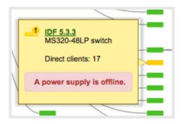
Learning which physical links in the network that are most heavily-trafficked is also effortless; simply hover over individual network links to learn statistics about that connection's negotiated speed, usage, and number of directly connected clients using it in the past day. This makes it simple to to diagnose physical bottlenecks in the network.
